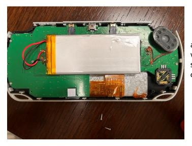
This is the back of the game console when taken apart. The main component of the back is a case which houses the battery which powers the other systems of the gaming console. The battery has a capacity of 2400 MaH
