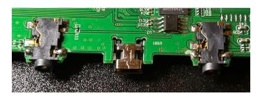
These are audio ports and the charger is in between the two, the audio ports allow for wired earphones to be plugged in or for an adapter cable that comes with the system to be plugged into a louder system, and the charger allows a cable to be plugged in to recharge the battery. The charger is a Usb mini A, which means it sends electromagnetic through inductive coupling to an electrical device which then gets stored in the battery allowing it to be used for longer uses.
