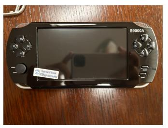
This is the Eliflame before I took it apart. There are four buttons on the left and right sides with a start and select button on the bottom right and a joystick near the bottom left. On the bottom there is a sim card port, and on the top of the system there is a sound button to increase and decrease the sound output from the console. Next to those are the audio jacks and a charging port. Finally, there is a power button on the side to turn the console on and off.
