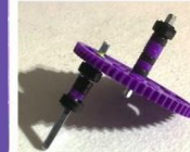
Prototype 3: Gear is not large enough for the dispenser. It slips and won't spin the wheel.
