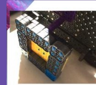
Prototype 1: Hard to attach to dispenser because it had to be at the exact correct angle to engage. Once engaged, it stayed nicely.
