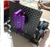
Prototype 2: Attached to dispenser easily but needed to be adjusted a bit. Tipped robot forward when the motor slowed down or the dispenser got stuck.
