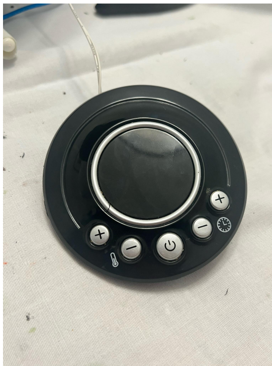
Step 10: In the top plastic cover, remove the snap on display screen for further analysis of the circuit board. (Figure 18 & 19, Left to Right)
