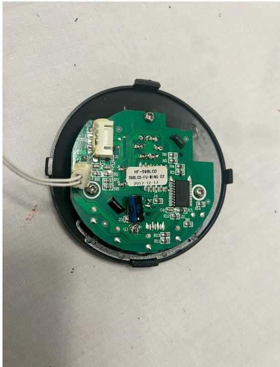
Step 10: In the top plastic cover, remove the snap on display screen for further analysis of the circuit board. (Figure 18 & 19, Left to Right)
