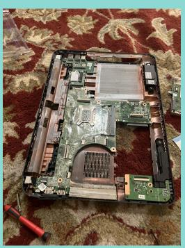
The Mainboard is where most of the mechanics of the computer is held. This board is underneath the keyboard (.on slide 3). It contains the motherboard, cpu, usb and microphone ports, and etc. The Mainboard is also the bottom half of the laptop.
