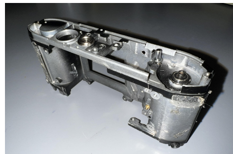
Figure 1.11: The frame of the camera once all of the components and parts of the camera were taken out. It is now a hollow piece with nothing inside.
