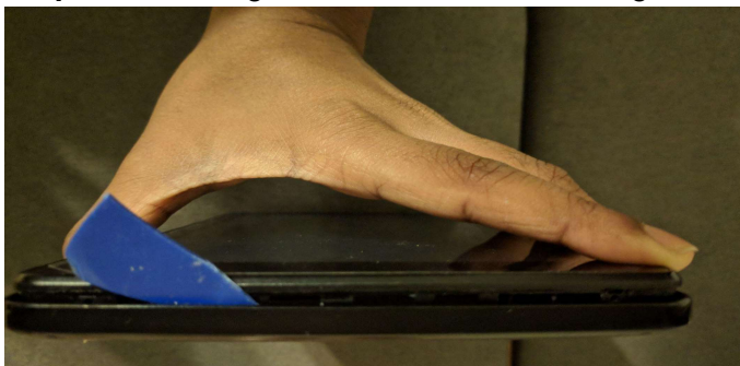
Broken plastic picks used to separate tablet
