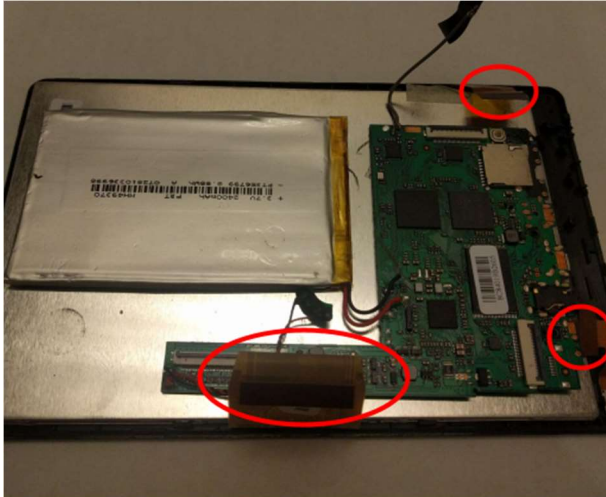
Removing the 3 flex wires
