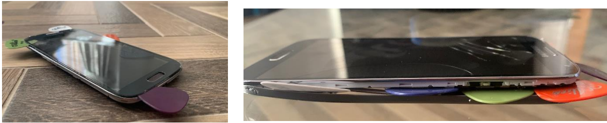
FIGURE 6 – GUITAR PICKS UNDER A GALAXY S4'S SCREEN
