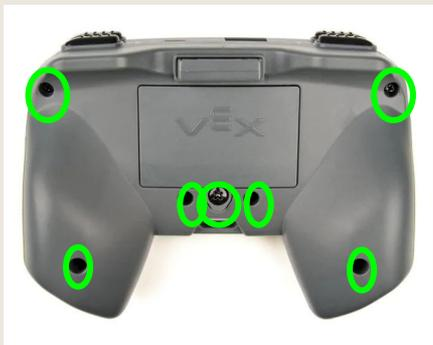
The controller has 6 screws and 1 For the battery compartment
