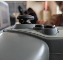
The buttons of the controller stick out of the faceplate and sit on caps inside laying on the PCB. The buttons themselves are long
