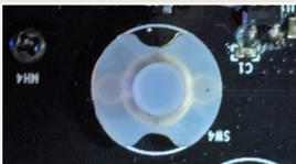
The Plastic caps are to push the buttons back up after being pushed down
