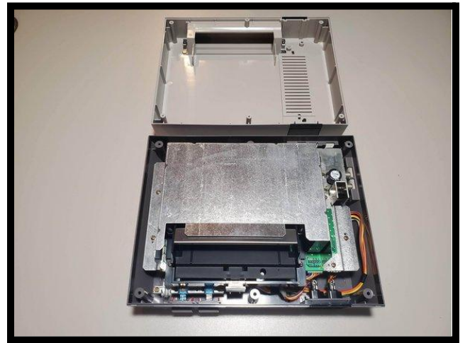
Figure 3.1.2: Take the top housing off the bottom of the system
