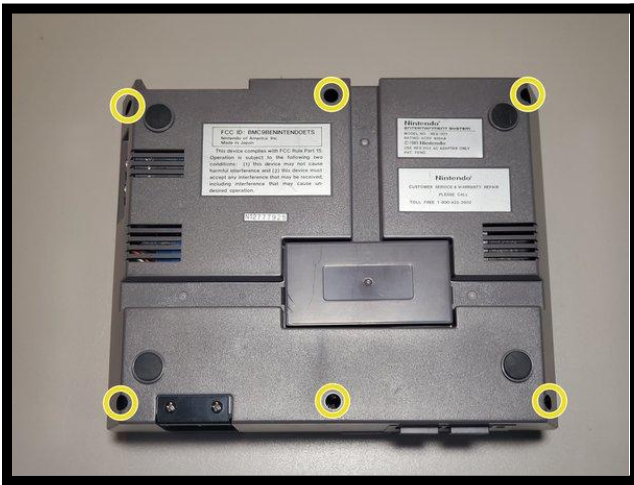
Figure 3.1.1: Remove the 6 screws shown
