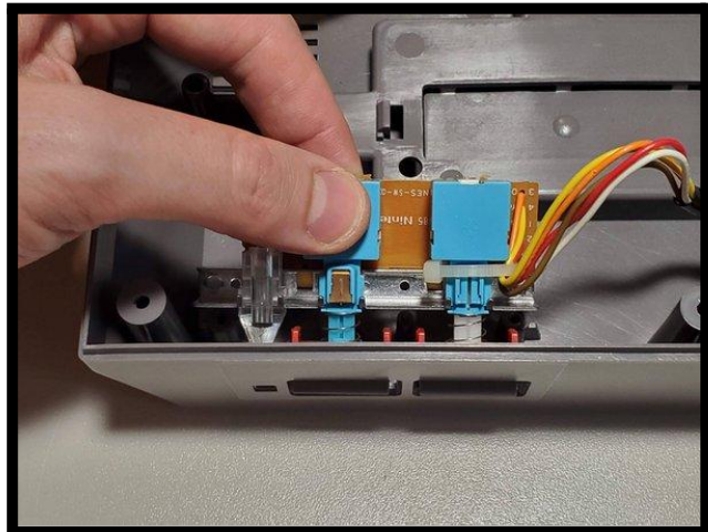
Figure 3.8.2: Remove the buttons from the housing
