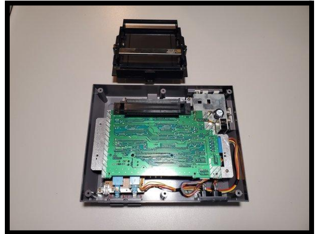
Figure 3.3.2: Remove the cartridge tray by sliding it towards the front of the system
