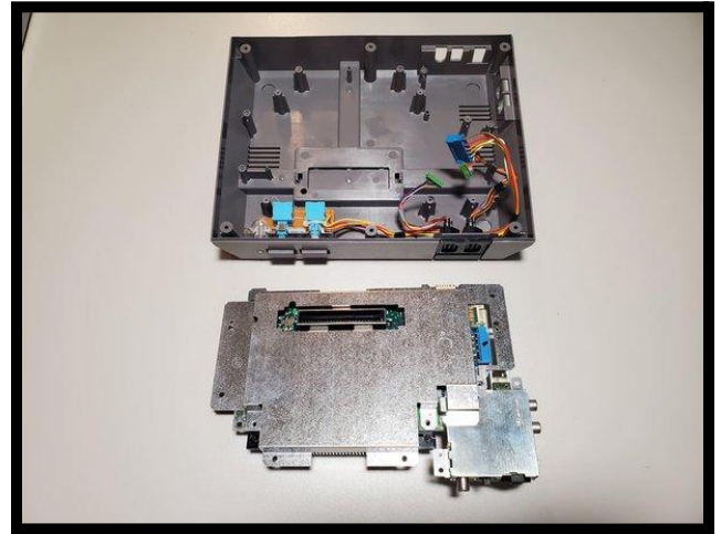
Figure 3.5.2: Remove the motherboard
