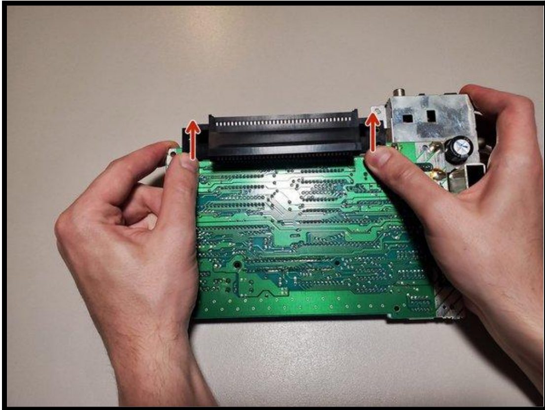
Figure 3.7.1: Push the 72 Pin connector off the motherboard as shown
