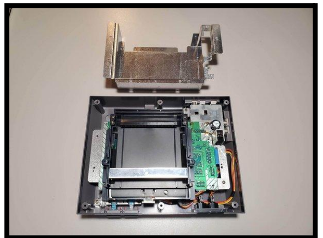
Figure 3.2.2: Lift the RF shield and place it to the side
