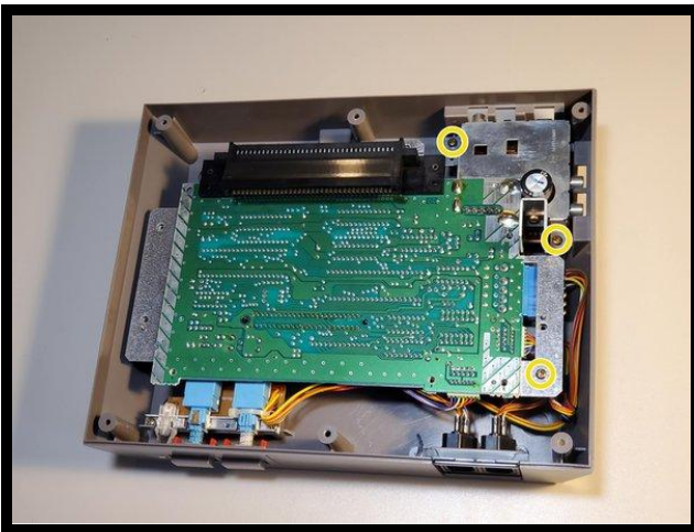
Figure 3.4.1: Remove the three screws shown
