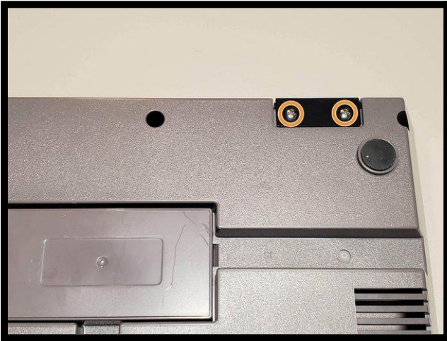
Figure 3.9.1: Remove the 2 screws
