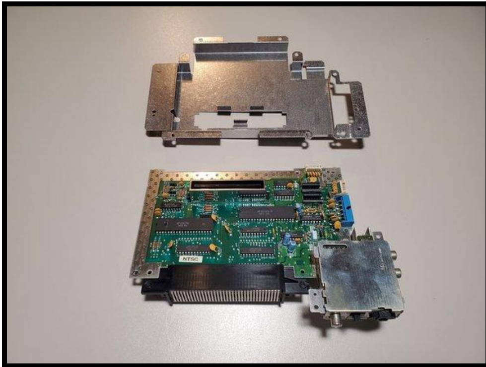
Figure 3.6.1: The shield is not held by screws. Remove the shield from the motherboard.
