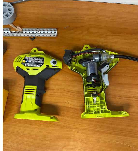
Figure 5: Outer shell removed
