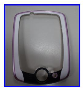
The front frame protects the motherboard and the screen. It contains buttons that control the screen, audio adjustment, and power.
