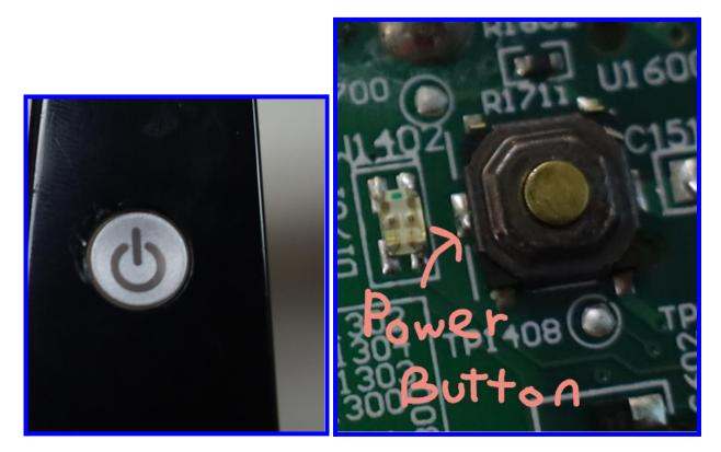
The power button controls if the LeapPad is on or off. When pressed, it turns yellow which allows the user to see that the LeapPad is now on.
