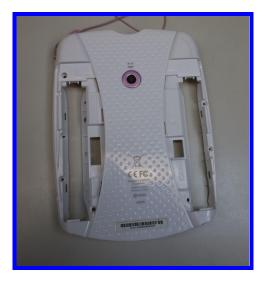
The back frame protects the motherboard and interior components of the LeapPad. It is a frame for the back camera and batteries. The frame has holes for ports and batteries. Additionally, it has a pen that
