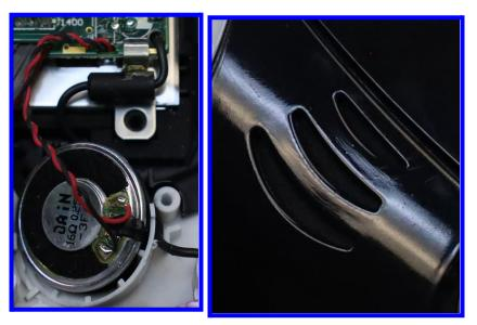
The speaker has a resistor of the value 16 ohms and will tolerate an electrical power of 0.25 Watts. The speaker receives input from the motherboard and outputs sound accordingly.
