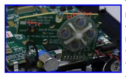
The button circuit board receives input from the exterior button and sends it to the motherboard through a ribbon cable. The button
