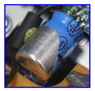
The capacitor stores electricity and can store up to sixteen volts. The size of the capacitor is 1000 micro Farad.
