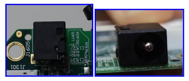
The charging port ensures that the LeapPad can charge to keep running. A charging cord is inserted in the charging port, which sends electric currents into the LeapPad. You can tell your LeapPad is charging when an indicator light turns on. It is placed on the motherboard right next to the USB port.
