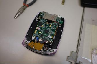
We removed the circuit board, which has a yellow backside in the picture above, behind the home and direction buttons. The circuit board had buttons that reacted to the pressure from pressing the external home and direction buttons. The button circuit board was connected to the motherboard with a ribbon cable that communicated the external input.
