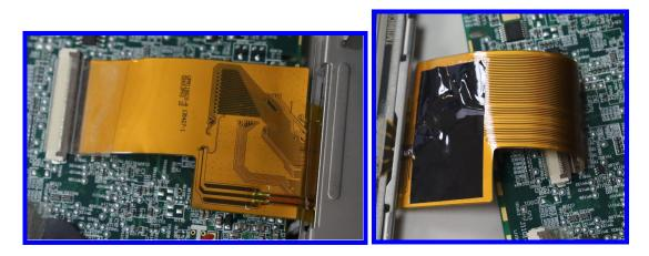
The yellow ribbon cable connects the screen and the motherboard. Information from the motherboard travels through the ribbon cable to the screen.
