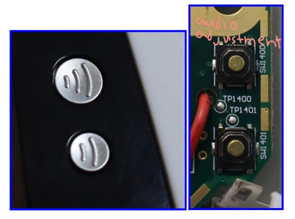
The two audio adjustment buttons increase or decrease the volume of the sound. It is found on the top right side of the frame.
