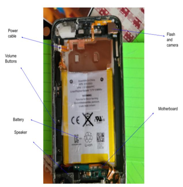
Next, we removed the logic board, which is the blue-green circuit present in the device. We found the speaker located on the bottom right and removed it. We also located the volume buttons and discovered that a deformed piece of metal was preventing them from working correctly. This helped us solve the mystery of the broken volume keys. Additionally, we removed the rear camera and found a snaking orange cable, which we concluded was the power cable.
