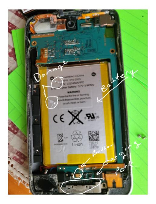
During our research on lithium-ion batteries, we also learned about the importance of safety measures when dealing with them. We found out that Lithium-ion batteries can be dangerous if they are damaged, as they may overheat, catch fire or explode. We also learned about the importance of proper disposal of these batteries, as they can be harmful to the environment if not disposed of properly.
