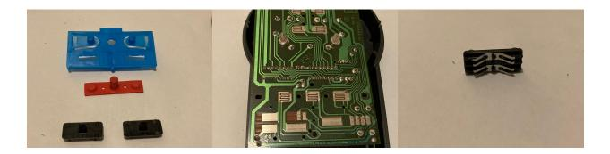
The buzzer used in this game was just a small piece of metal, sitting in a plastic holder. When put together, 2 contacts of metal from the circuit board touched the piece of metal sitting in the plastic holder. The plastic holder also turned out to be a light diffuser.
