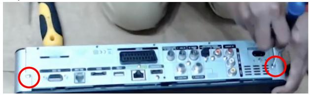
Step 2: Remove the two screws indicated below in red circles
