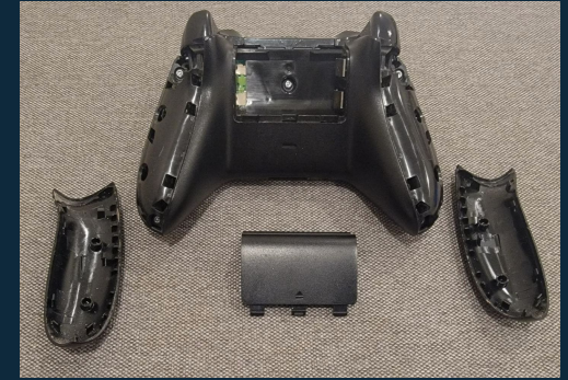
Removed handle and battery covers
