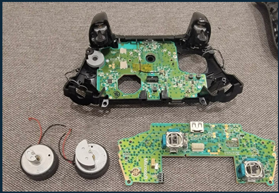
Removed daughter board and rumble motors
