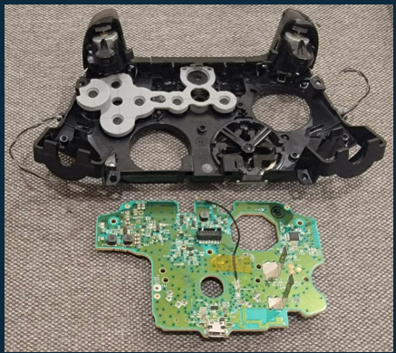
Removed motherboard from mid frame assembly
