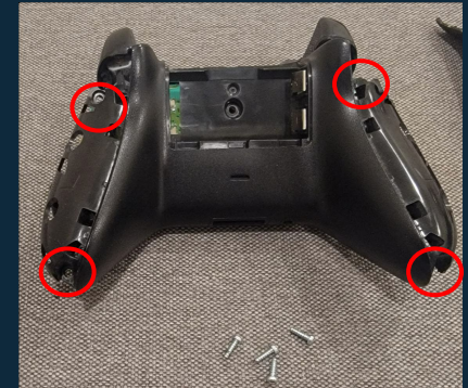
Unscrewed four T8 torx screws
