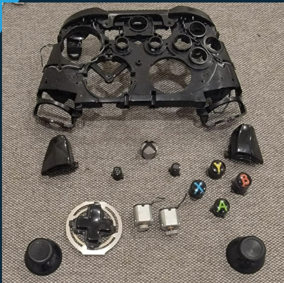
Removed action button covers, joystick and bumper covers and small rumble motors
