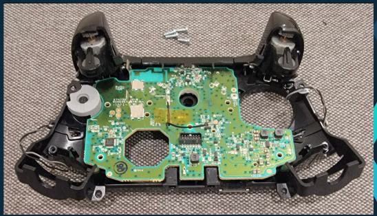
Unscrewed four T6 torx screws from motherboard
