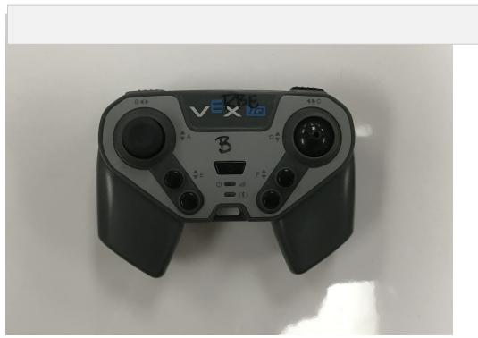
Before deconstruction, we initially knew what the problem was, but we didn't know how it was created. The problem was that the charging port wasn't working so that made the controller unable to be used. Whenever we picked up or worked on the remote at all we heard an object moving inside, meaning that it was loose. Once we got to the part where the loose object was, we realized that it was the charging port that "wasn't working".
