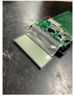
How does the calculator get power in order to function? It uses solar cells that collect solar energy. If you look at the front of the calculator, you will see a tiny rectangle above the screen. This rectangle gathers solar energy (positive charges) and delivers it through our red wire so that it can recharge the lithium battery and cycle through the process that I explained earlier.
