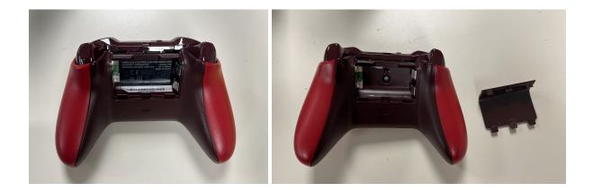
We decided to start with the easiest part to remove, which is the battery cover. Then the sticker, finding a screw and removing that with the Torx 8 screwdriver.
