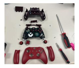
We used a flat-head screwdriver to lift the metal ring around the plastic hook. We removed all the buttons and controls to finish off and go as far as we can to deconstruct the controller.
