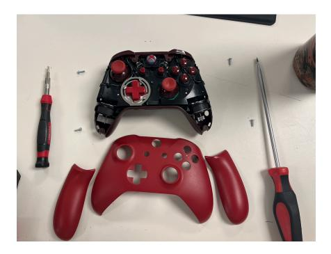
We removed the screws using the Torx 8 Screwdriver and took off the faceplate of the controller.
