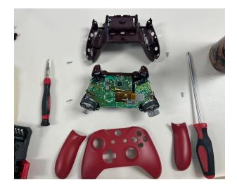
We realized the back cover of the controller could be wiggled off. We slid a flat-head screwdriver underneath the plate next to the buttons and removed the cover off the top of the controller.
