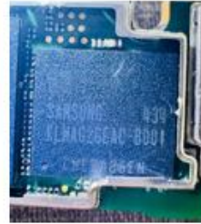
SAMSUNG KLMAG2GEA C-B001 Memory/RAM
