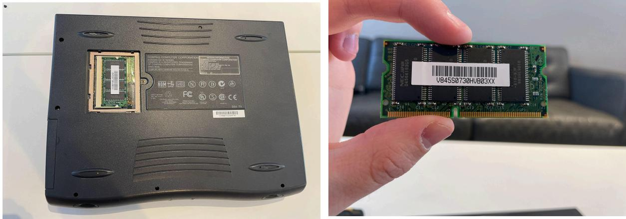
The RAM was the easiest to access, so we documented it first. The role of RAM is to temporarily store data from a program being used. RAM capacity is measured in gigabytes, however, RAM is not storage.
