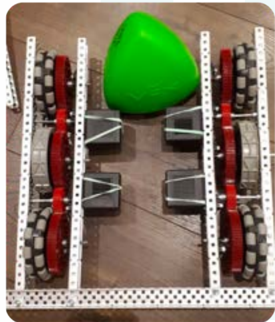
FIGURE #15: V1 VS V2 DRIVETRAIN COMPARISON, NEW SLOT FOR TRIBALL, QUICK SWITCH MOTORS, IMPROVED GEAR RATIOS
