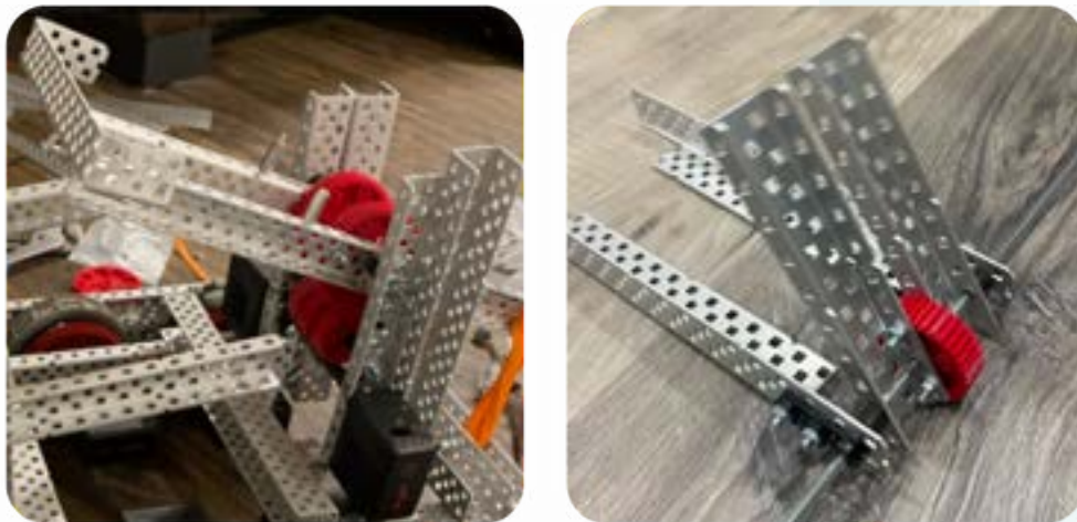
FIGURE #9: EARLY STAGE BUILD OF THE CATAPULT BASED OFF THE CAD MODEL TO TEST FUNCTIONALITY
