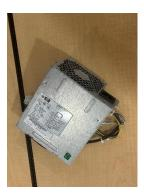
The power supply unit (PSU) it's a hardware that changes ac current to dc current and distributes it to the rest of the components.
