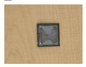
The central processing unit (CPU) is better known as the brain of the computer. It is the control unit that processes every computer operation. The CPU is made out of microprocessors that have the circuitry and logic to process whatever task you put on it. Depending on the CPU some might even have display capabilities and don't need a graphics card.
