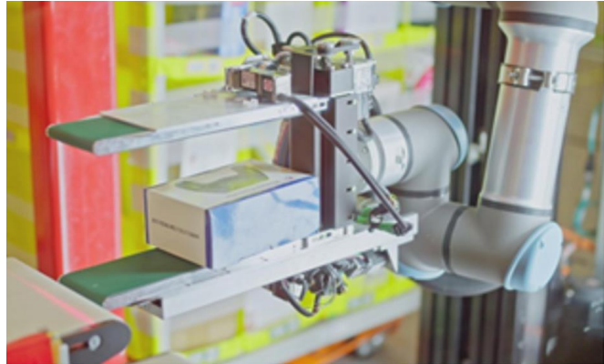
The Stow robot's EOAT after being built
