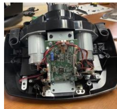
Fig. 6: Wheel Base with Top Off
