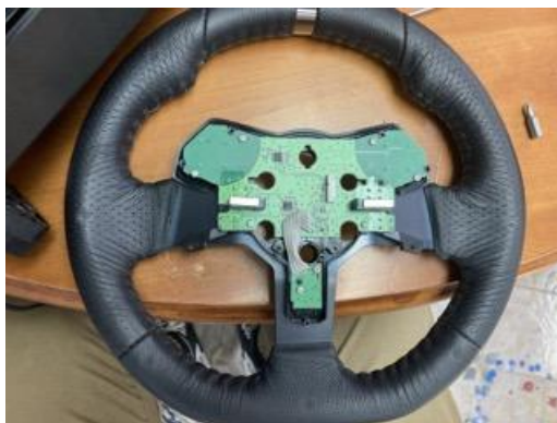
Fig. 5: Wheel Itself Detached from Body
