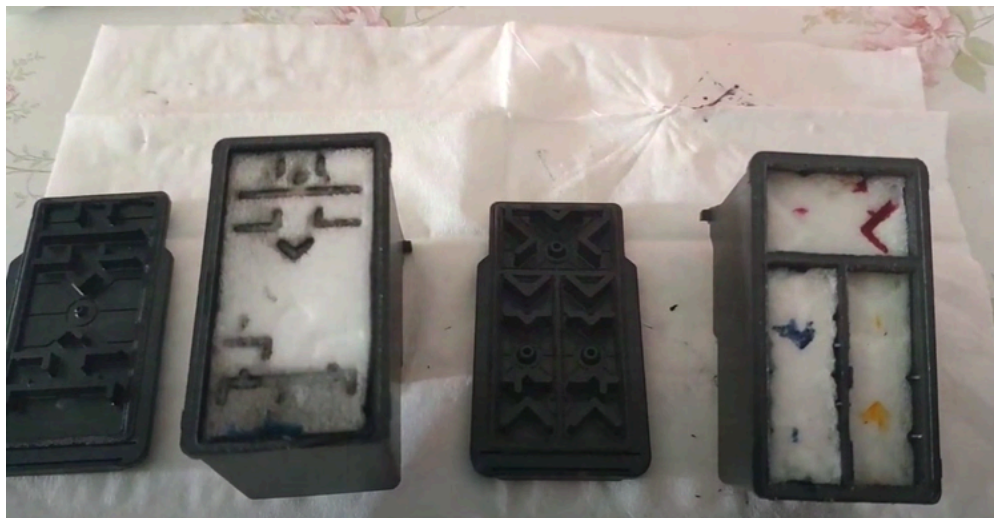
Figure 6.4. The insides of the ink cartridges (black on the left and cyan, magenta, and yellow on the right). Each cartridge has separate compartments for sponges filled with ink of each
