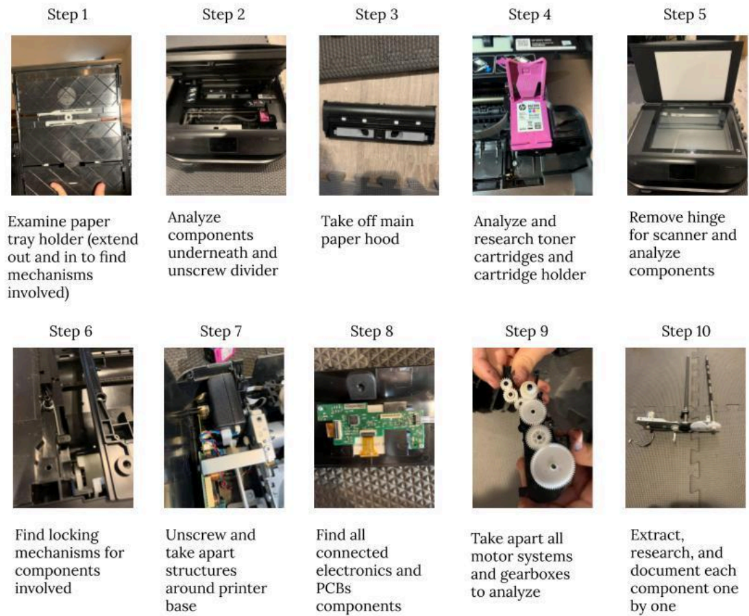
Figure 4.1. How to disassemble the printer and analyze components. View it here .
