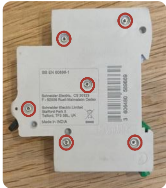
Fig 2.2, Rivets on the Schneider Electric MCB (Circled in red.)
