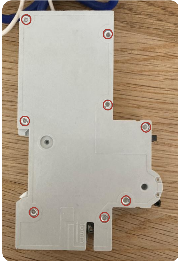
Fig 2.1, Rivet holes on the Wylex 16A Type B RCBO (Circled in red.)
