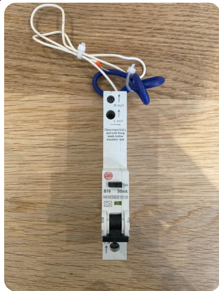
Fig 1.1, The Wylex 16A Type B RCBO that we reverse engineered.
