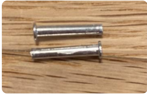
Fig 2.6 The locking pins found on both breakers.
