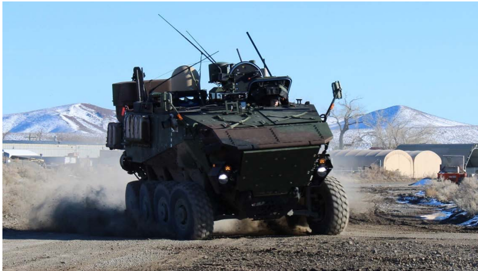
The prototype Advanced Reconnaissance Vehicle made by General Dynamics Land Systems.
