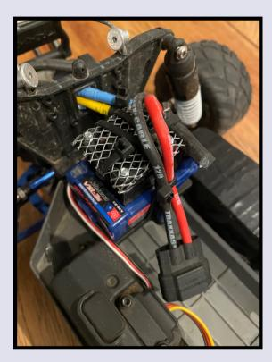
Electric Speed Controller (ESC)
