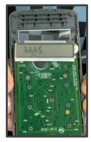
The first noticeable thing is the LCD screen. LCD stands for liquid crystal display. The LCD screen uses the light modulating properties of liquid crystal combined with polarizers to display an image.
