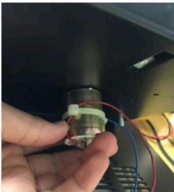
Step 5: Removed the motor
