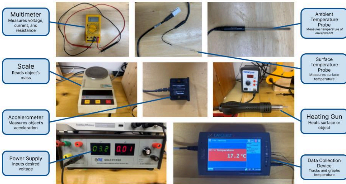
Figure 3: Labeled equipment used with descriptions
