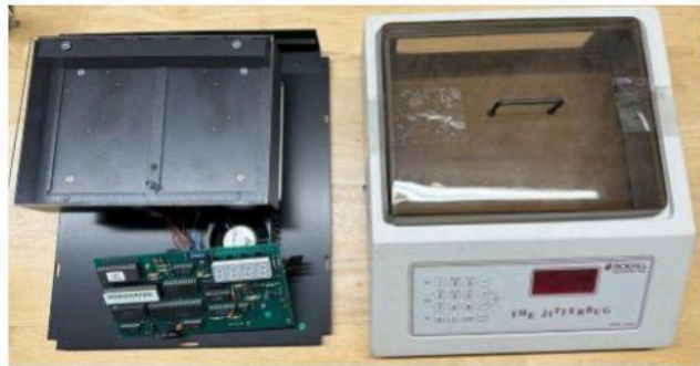
Step 1: Removed the exterior casing
