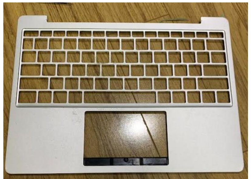
Figure 74 – Front of keyboard/trackpad shell with trackpad and keyboard removed
