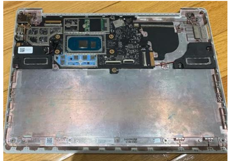
Figure 56 – Surface Laptop Go with plastic shieldings removed
