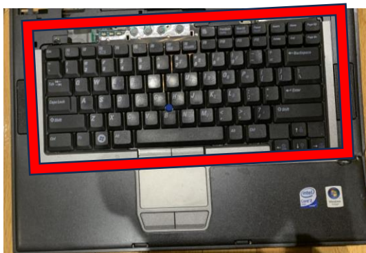
Figure 10 – Dell Latitude with button strip above keyboard removed
