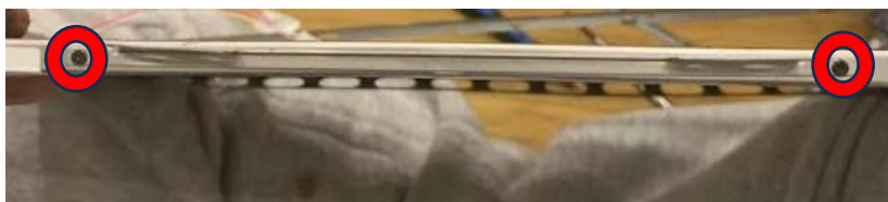
Figure 29 – Dell Latitude D830 Screen with bottom screws outlined in red
