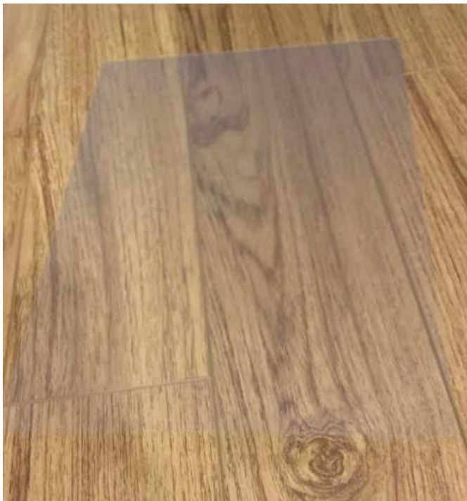
Figure 67 – Transparent layer found between backlight and Liquid Crystal
