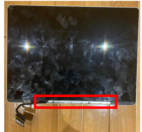
Figure 60 – Surface Laptop Go screen with Wi-Fi antenna source removed (location outlined in red)
