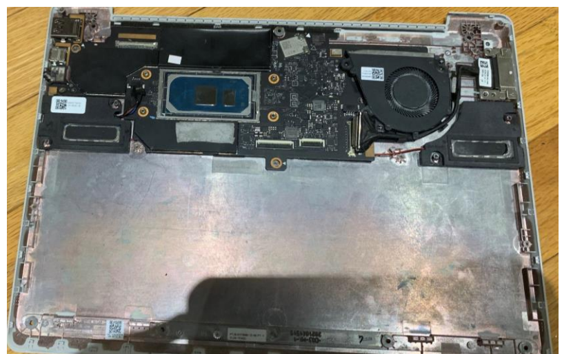
Figure 54 – Surface Laptop Go with heatsink and thermal paste removed
