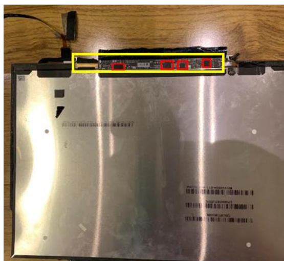
Figure 64 – Surface Laptop Go screen (back view) with LCD Controller Board outlined
