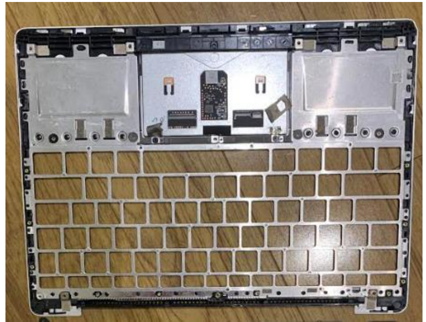
Figure 72 – Back of keyboard/trackpad shell with keyboard removed
