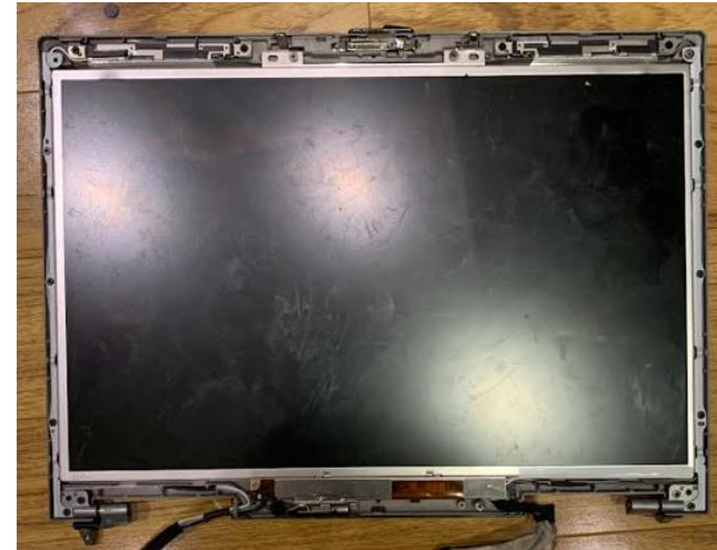
Figure 22 – Dell Latitude D830 Screen with bezel removed
