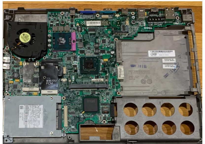
Figure 16 – Dell Latitude D830 with heatsink and PC Card Slot removed
