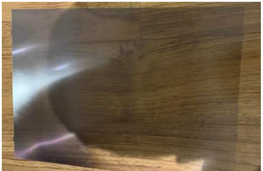
Figure 68 – Polarizing layers found between backlight and Liquid Crystal
