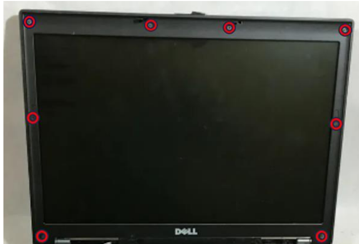
Figure 21 – Dell Latitude D830 Screen with screws on bezels outlined in red
