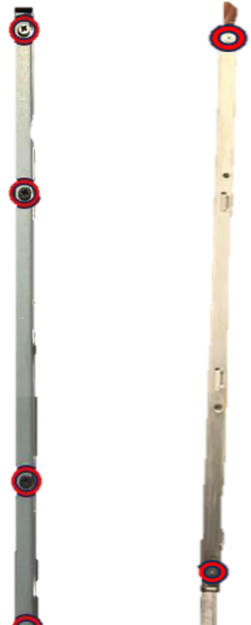
Figure 28 – Dell Latitude D830 Screen with side screws outlined in red
