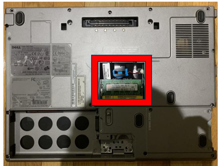
Figure 9 – DELL Latitude D830 with back panel removed
