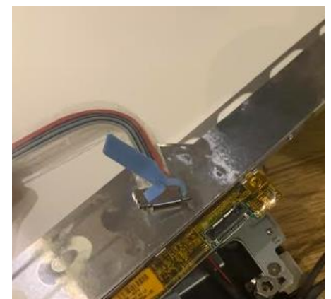
Figure 26 – Dell Latitude D830 Screen with connection to inverter unplugged
