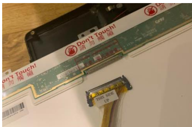
Figure 25 – Dell Latitude D830 Screen with connection to LCD Controller Board unplugged
