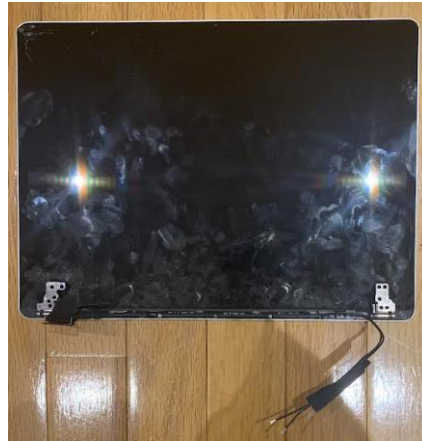
Figure 59 – Surface Laptop Go screen with Wi-Fi antenna source shielding removed
