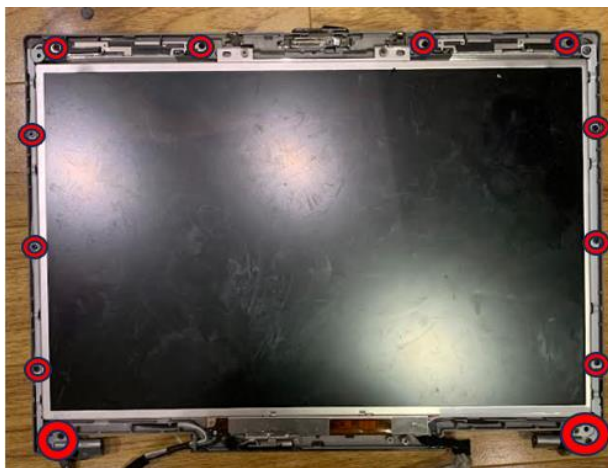
Figure 23 – Dell Latitude D830 Screen with screws attaching screen to shell outlined in red
