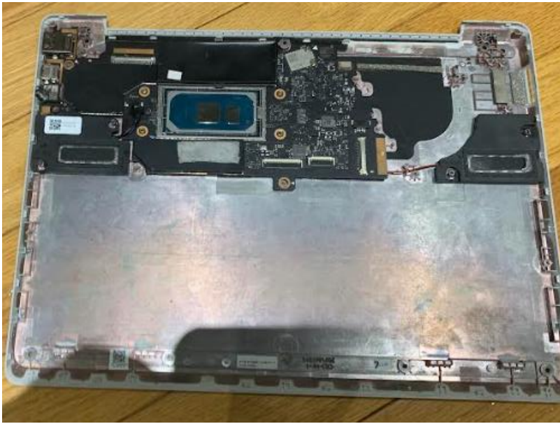
Figure 55 – Surface Laptop Go with Surface Connect (or Surfink) port removed
