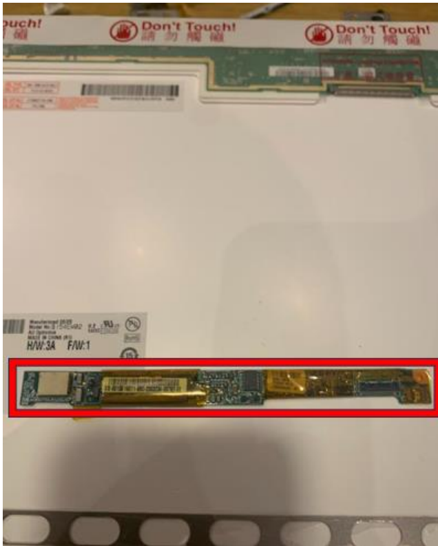
Figure 27 – Dell Latitude D830 Screen with inverter removed and outlined in red
