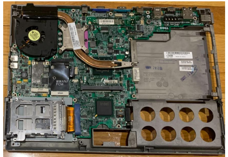
Figure 14 – Dell Latitude D830 with modem and PC Card removed
