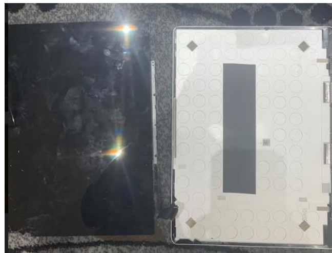
Figure 62 – Surface Laptop Go screen (left) separated from its shell (right)
