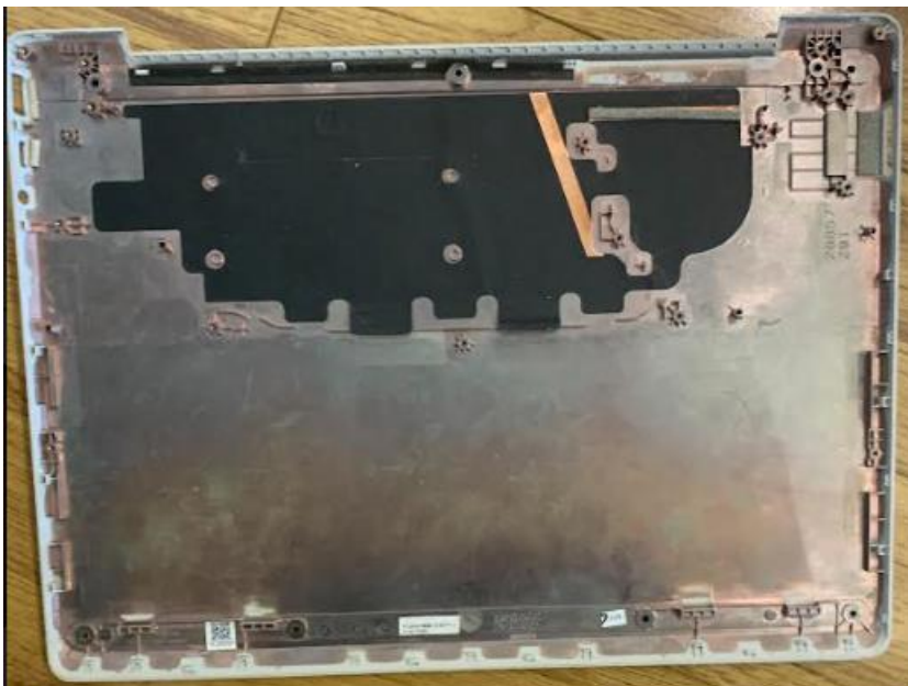
Figure 57 – Surface Laptop Go with motherboard and speakers removed
