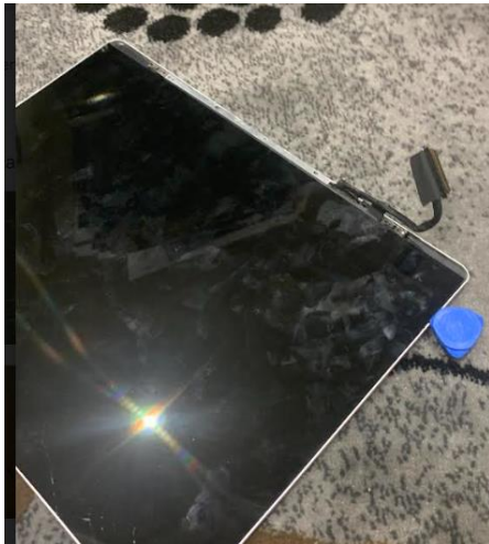
Figure 61 – Surface Laptop Go screen with plastic triangle removing the screen from its shell
