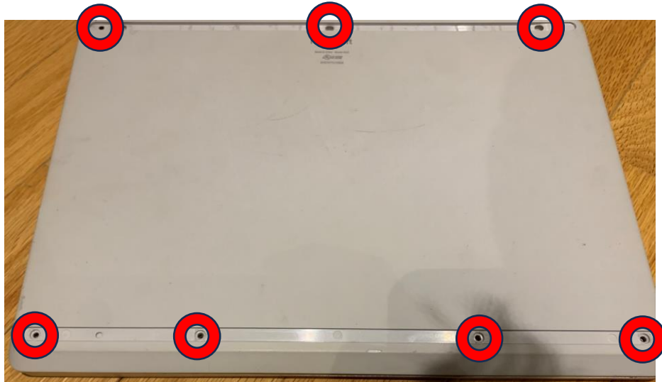
Figure 51 – Surface Laptop Go bottom with screws outlined in red
