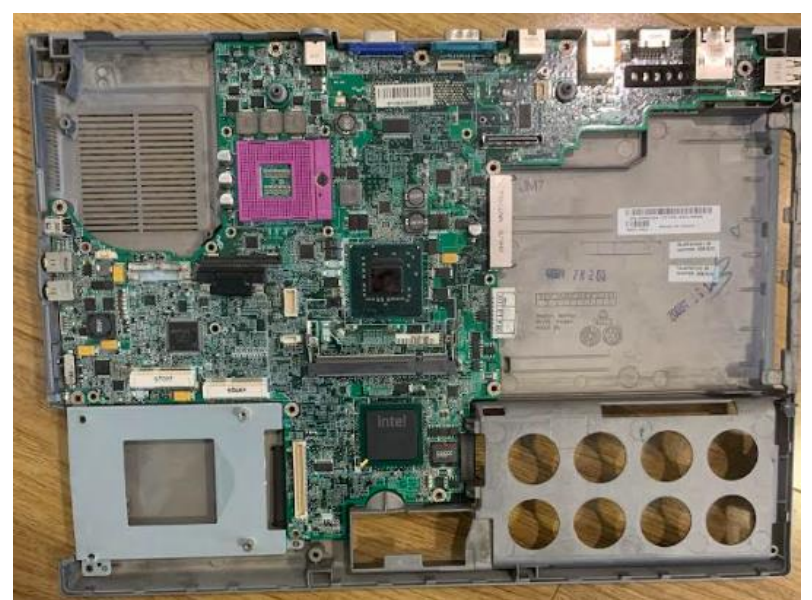
Figure 20 – Dell Latitude D830 with Wi-Fi card and HDD removed
