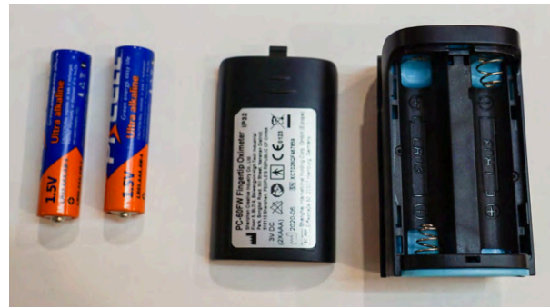
Step 1: Remove all batteries
