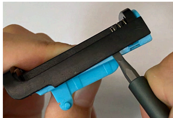
Step 5: Remove the bottom lid/Battery holder
