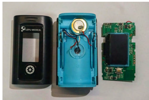
Step 3: Remove the motherboard
