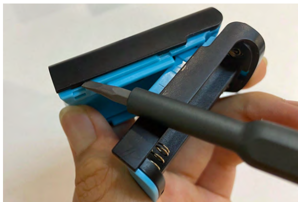
Step 2: Remove the top lid of the oximeter
