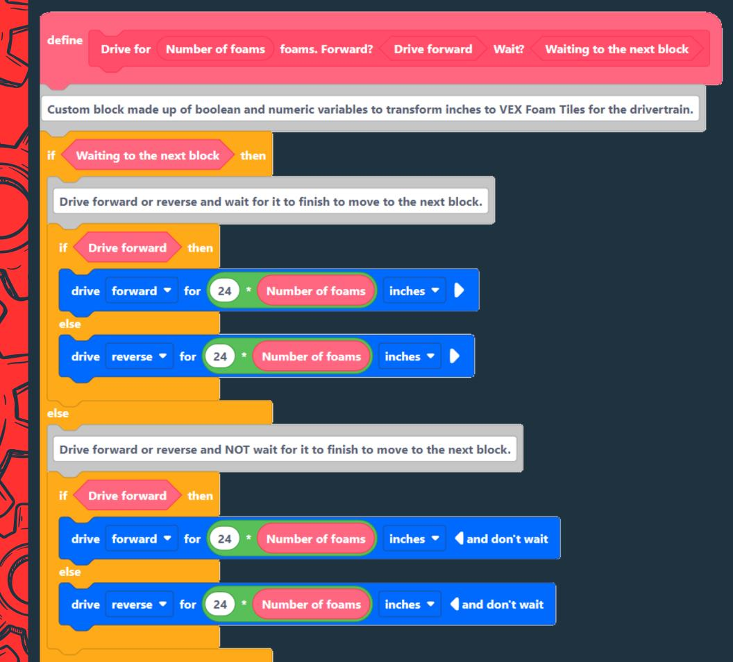
Milimiters? Inches? Nah.. We use a custom block for the robot to handle distances in foams. In this way, we have a more visual division of the field that makes it easier for us to calculate distances when programming. This block works by numerical and boolean values, as well as having all the capabilities of a normal driving block. It's a simple, effective, and functional way to make our robot move.
