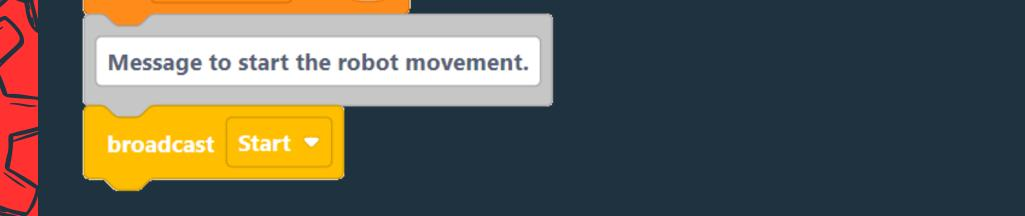
These blocks are used to set all speeds, variables, and configurations before the robot and its mechanisms are set in motion to avoid bugs. We use the message block as a signal to trigger various simultaneous processes, such as movement and the automatic system. This does not cause a delay for the robot to start moving.
