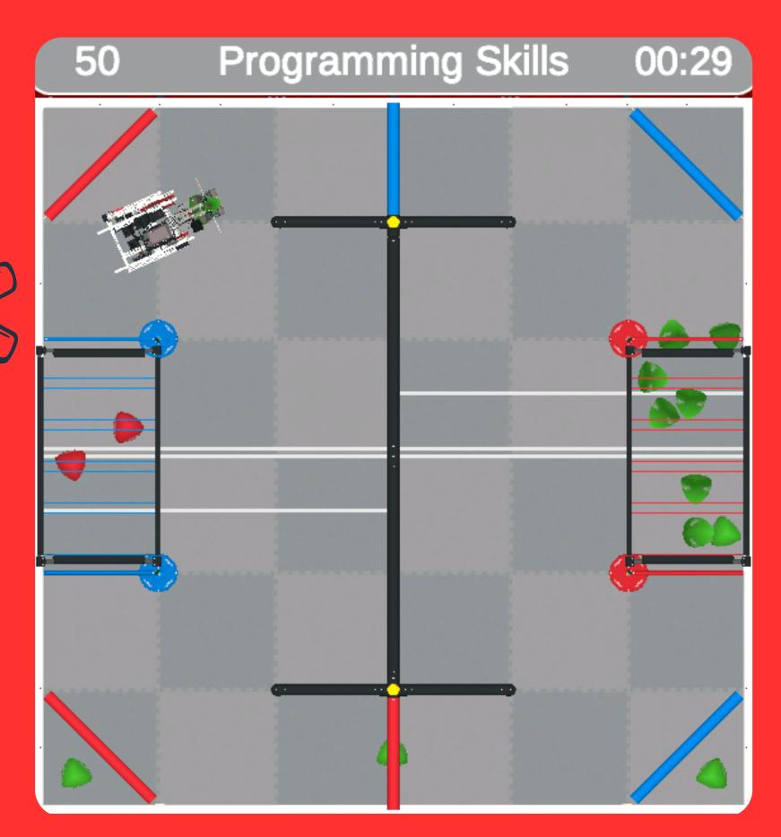
The robot headed to the LoadZone1 and is getting ready to the Repeat section. Here on the repeat section the arm raises to shoot farther.
