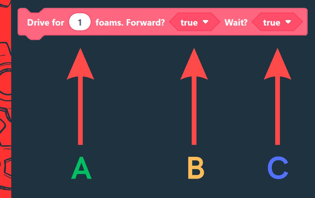
A. Numeric variable used to indicate how many foams the robot will traverse. (Supports decimal
