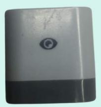
This is colour sensor we can use, so that our robot can sort trash bags by colours
