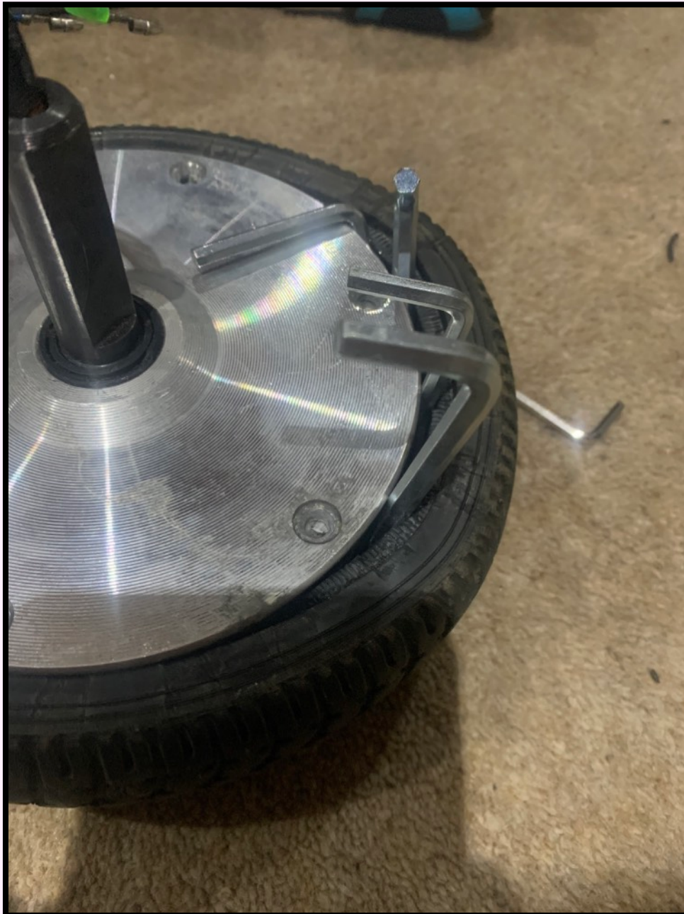
Figure 21: Using a thick metal screwdriver, we were able to pry open gaps between the tyre and the frame to insert Alan keys into the gaps along the whole circumference of the rim. In this way, we managed to take off the tyre.
