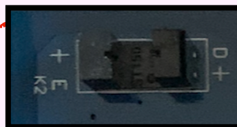
Figure 16: The IR sensor which can be seen on the opposite side when disassembled.
