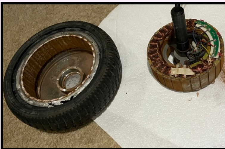
Figure 24: The motor separated from the rim.
