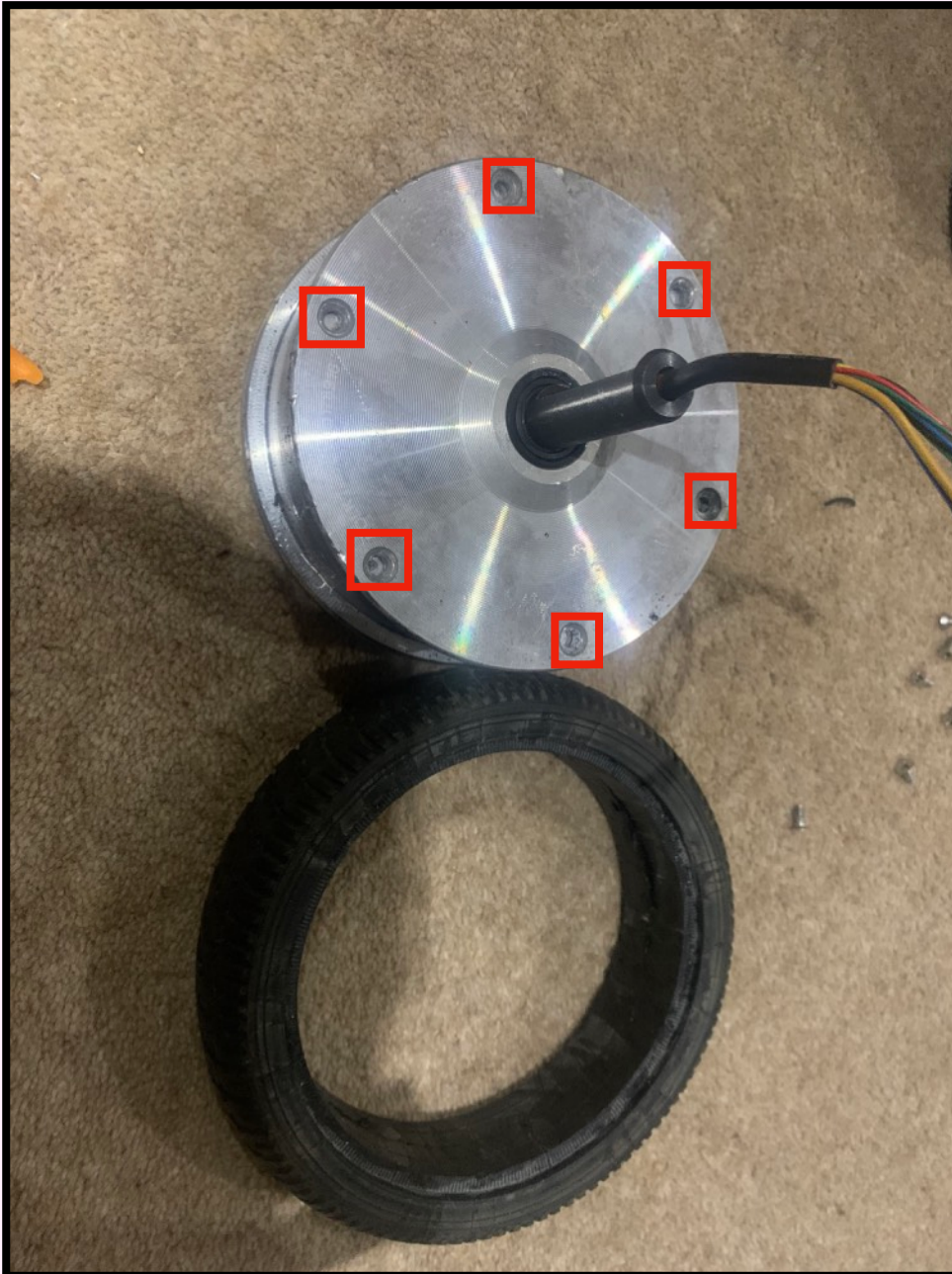
Figure 22: Tyre separated from the rim.
