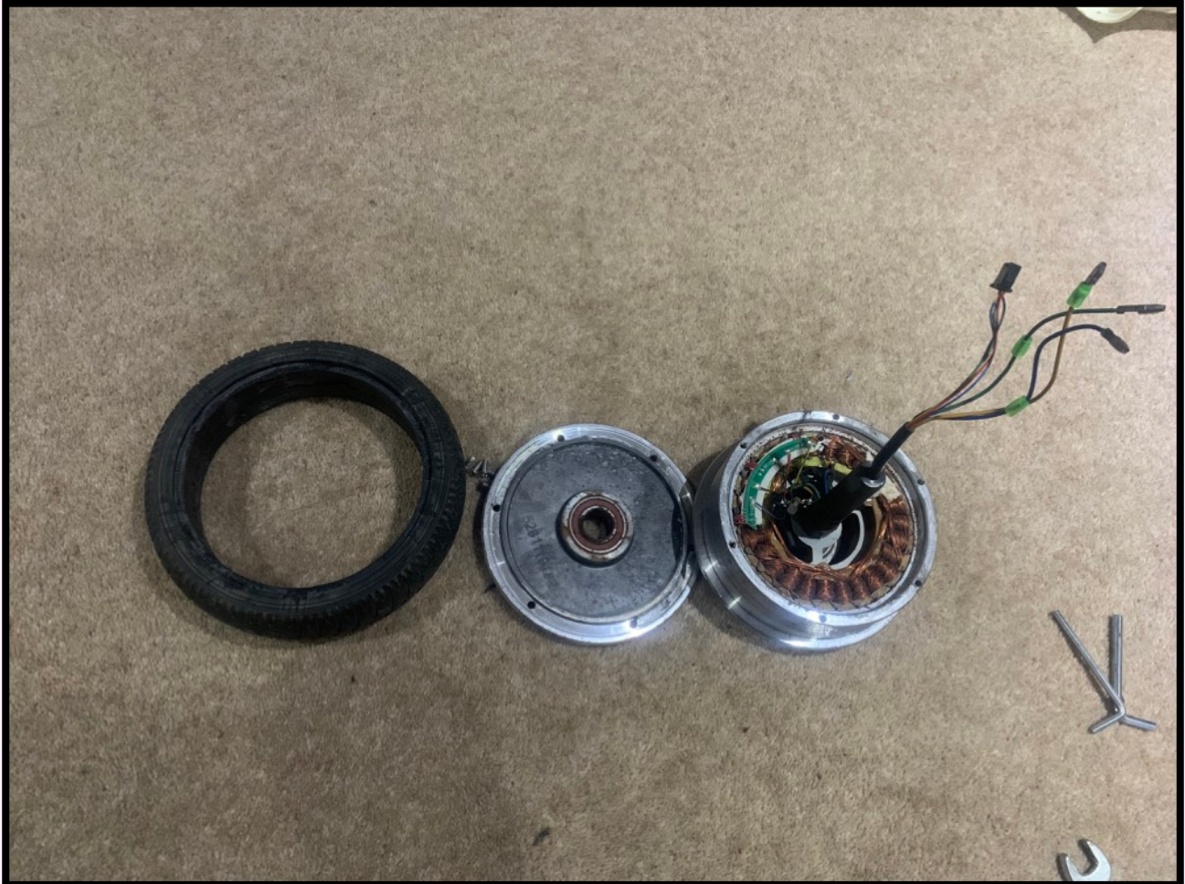
Figure 23: The three components of the wheel separated.
