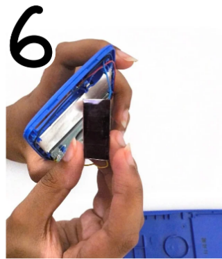
6. The solar panel is another source of power that we detached from its frame.
