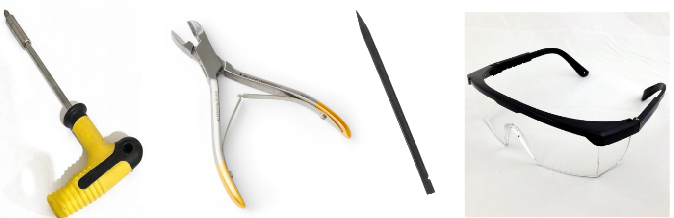
Figure 4: These are the tools we used in our disassembly process. We used a screw driver, a wire cutter, a spudger to separate parts, and goggles for safety.
