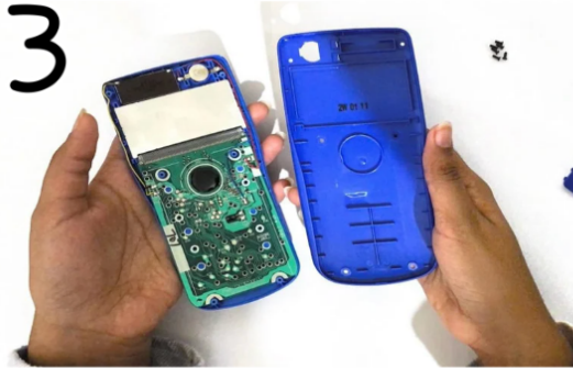
3. We separated the back cover from the rest of the calculator.
