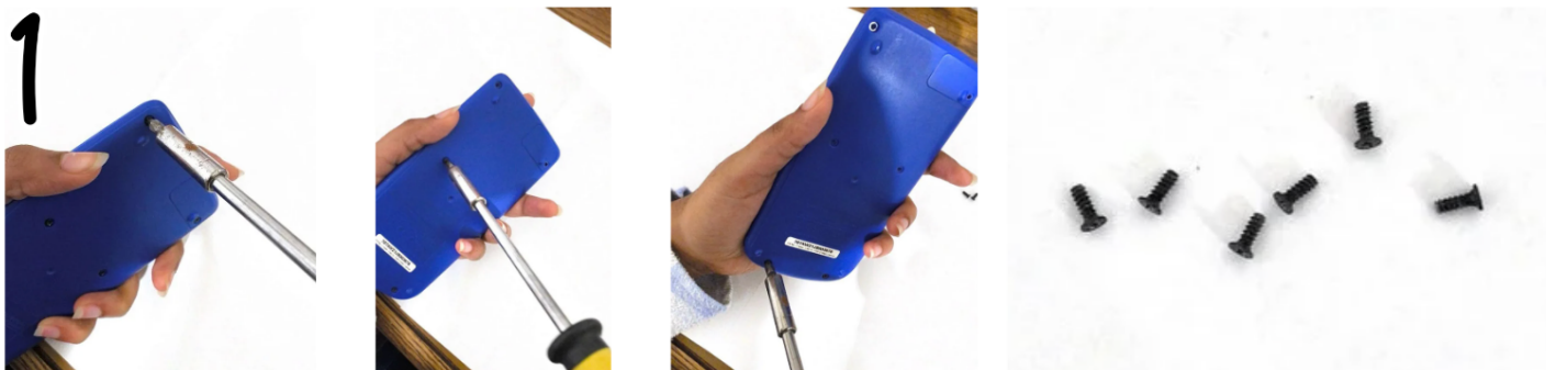
1. We removed the 6 screws on the back of the calculator using a Phillips screw driver to separate the frame from the rest of the calculator. To the right is a zoomed in view of the screws we removed.
