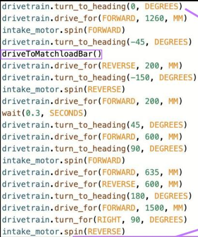
I have used the turn to heading command here because the conditional logic prior to this does not guarantee the heading the robot will be in.
