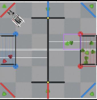
We have utilised two cycles of matchloads, this is because this cycle is very time-taking, with one cycle taking approximately 5 seconds. The matchloads consistently land in the tile which has been highlighted. This allows us to later score them when we get to that side of the field.
