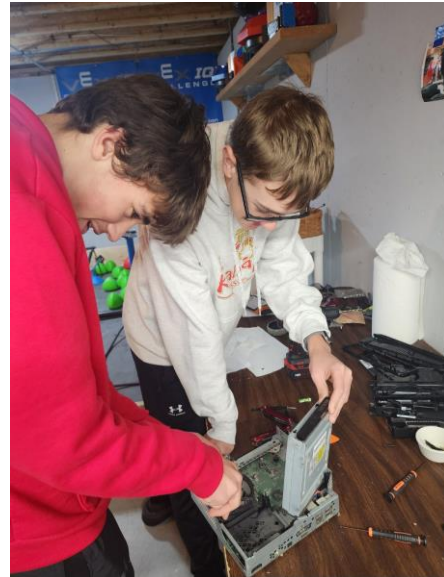
Figure 5 – Removing the Optical Drive
