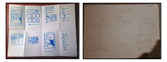
Left: example of Crazy-8 sketching. Right: our own robot design ideas. We use this step in our robot design process, sketching many different possible robot designs with different functions. The sketches are rough without intricate details, using a broad range of ideas. This helps us identify possibilities for our final design which is useful for building the optimal robot.
