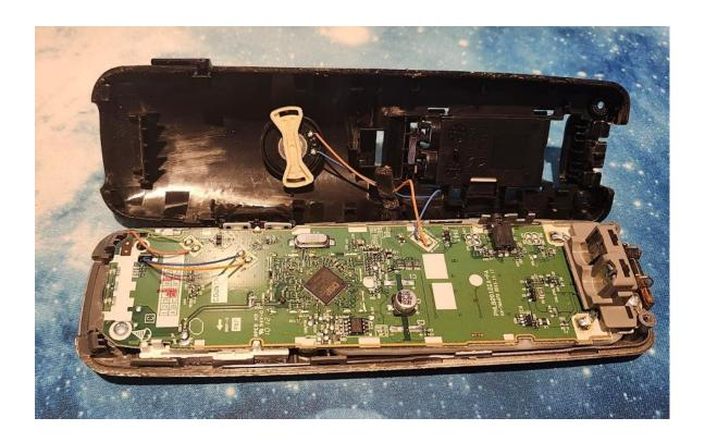
The motherboard is a printed circuit board (PCB) that houses, connects, and delivers power to every component of the handset. It was specially designed for this device and uses different connectors to interact with each component.
