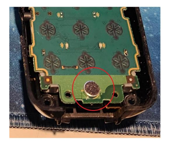
The microphone collects the speech input from the user to be interpreted and transmitted from the handset to the landline base. It works by using a diaphragm to pick up sounds which are converted into electrical currents via a magnet that alters the current of a nearby coil.
