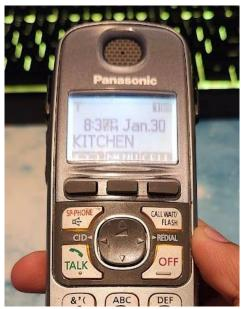
The screen displays data to the user about the system including caller information, date & time, battery level, and signal strength. It works using a backlit Liquid-Crystal Display (LCD) with electrodes that when charged, allow light to pass through a polarizing filter, creating an image on the screen.
