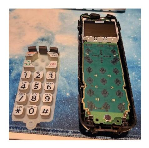
The keypad circuit board uses a series of physical buttons connected directly to the back of the motherboard that provide the user a method to interact with the handset. It uses push-buttons as inputs which are communicated to the motherboard and microprocessor that determine what the system will output.
