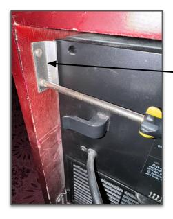
STEP 1: Remove the screws from the back panel (8 screws total).
