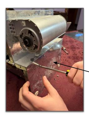
STEP 15: Unscrew the back fan panel and remove it from the rest of the heater.
