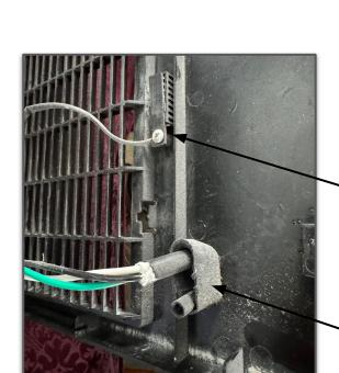
**STEP 9**: Unscrew ground from the back panel.
