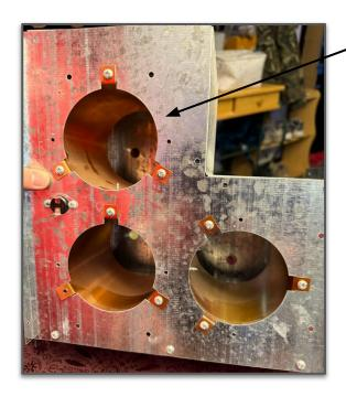
**STEP 18**: Remove the inner left side panel (9 screws total). There are three cylinders that are attached to the left side panel.
