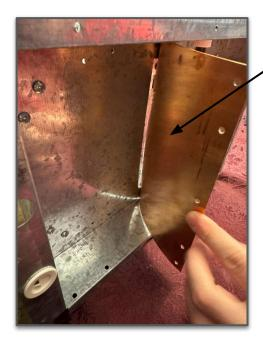
STEP 13: Remove the copper curved panel from the front (2 screws total).
