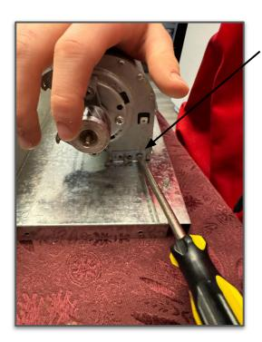
**STEP 16**: Remove fan motor from the inner back panel (6 screws total).
