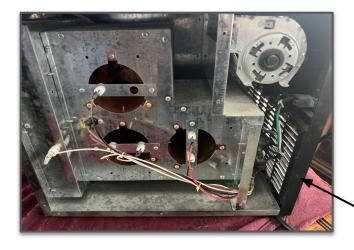
**STEP 6**: Unscrew front and back panels (12 screws on front, 6 screws on back). The front panel is attached to the bottom panel.
