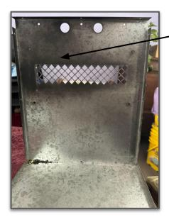
STEP 11: Unscrew the bottom panel (which is part of the front panel). Note: the backside of the front panel was a lot darker than the other side. It almost looks burned.
