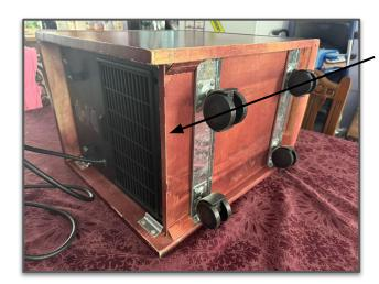
**STEP 4**: Remove the vent cover and filter.
