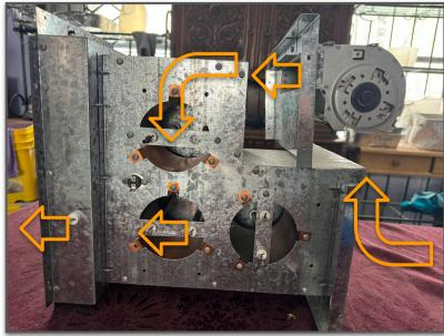
Third, I learned how the safety feature works. When the heater tips over, the free-rotating metal piece hits a limit switch. This limit switch turns the heater off so nothing catches on fire.
