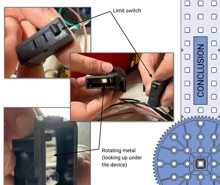
Rotating metal (looking up under the device)
