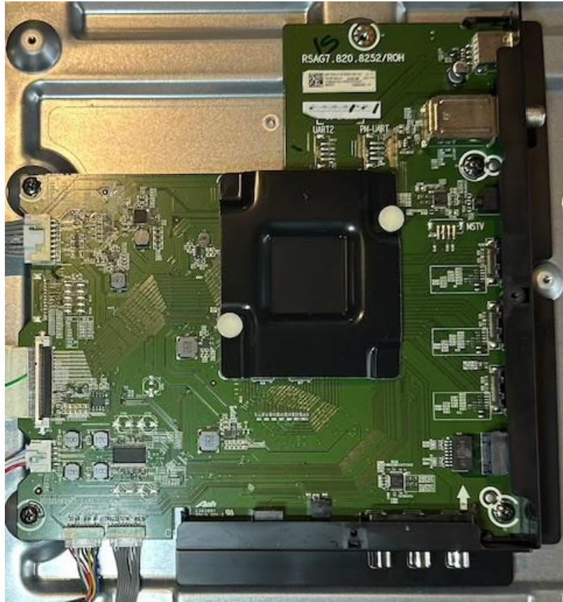
Main Board (RSAG7.820.8252/ROH)
