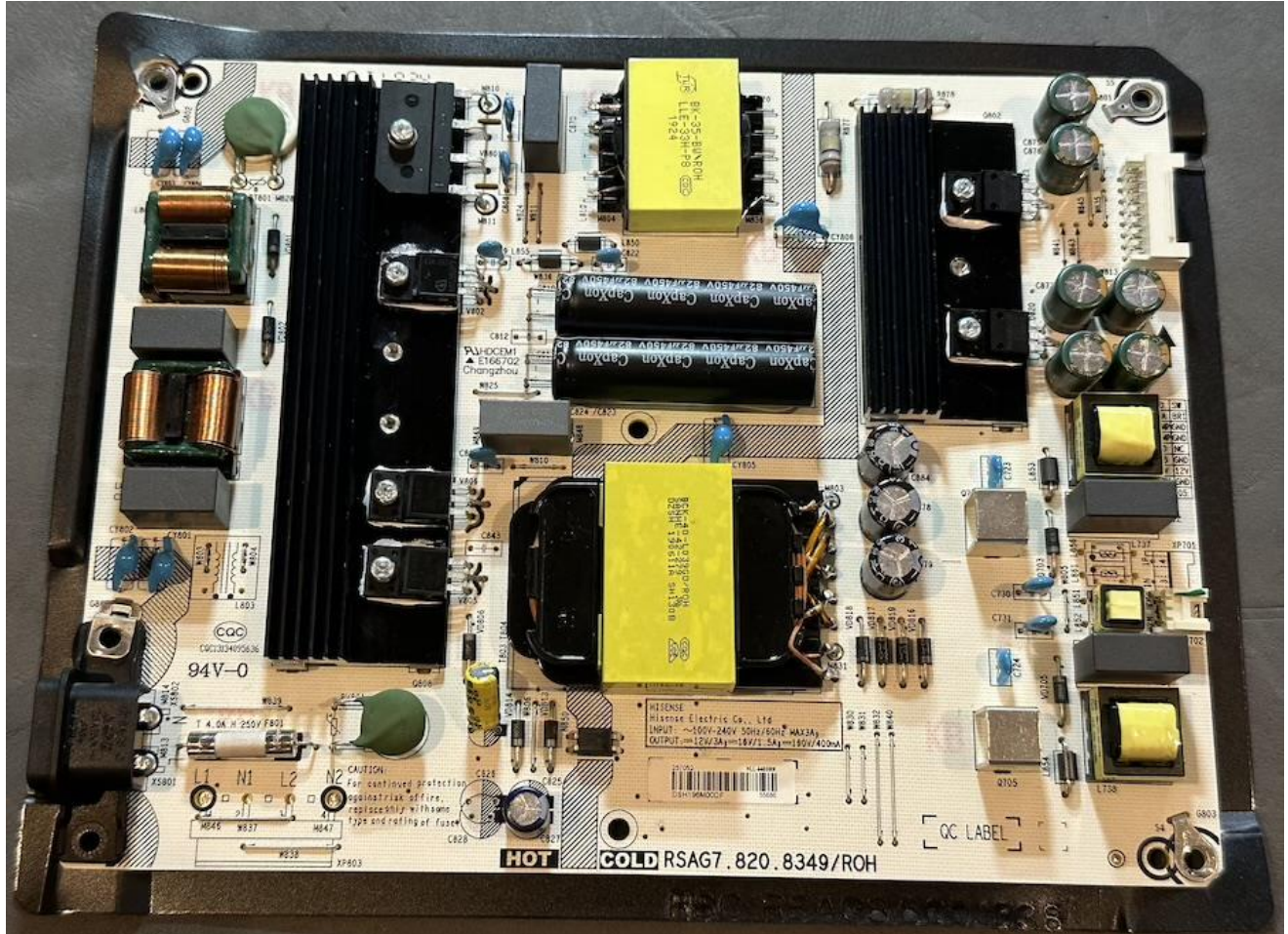
RSAG7.820.8349/ROH Power Board
