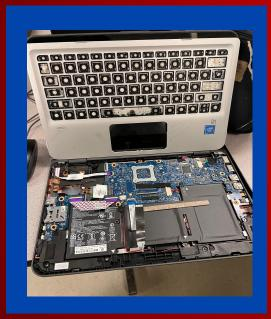
First and foremost, in order to examine the underside of the keyboard itself, we had to remove it from the laptop. We accomplished this through pinpoint force, and precise leveraging, with the assistance of tools.
