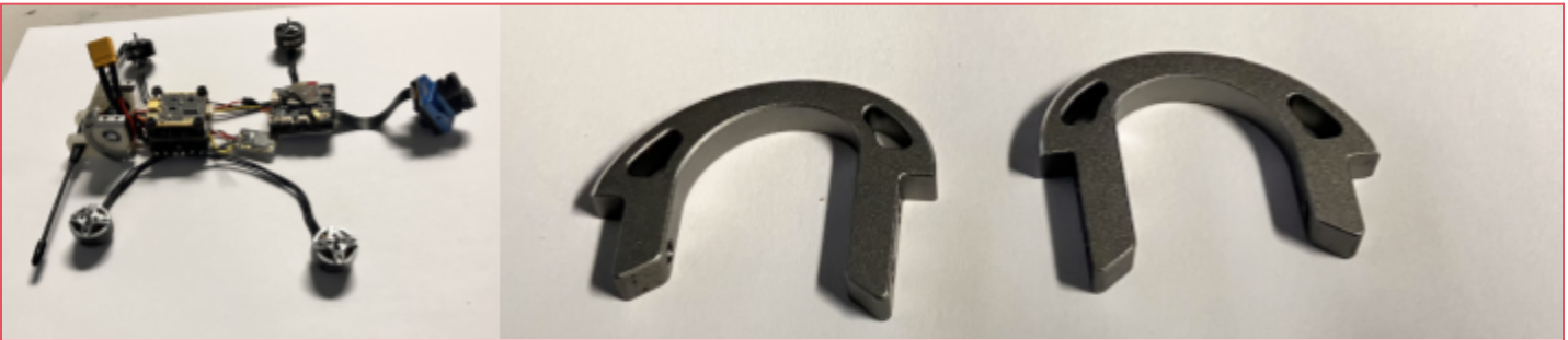
Step 5: Deconstruct camera structure/frame and dual camera
