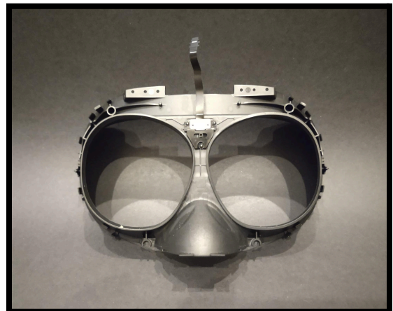
Figure 3.2 - Removal of the eyepiece trim.
