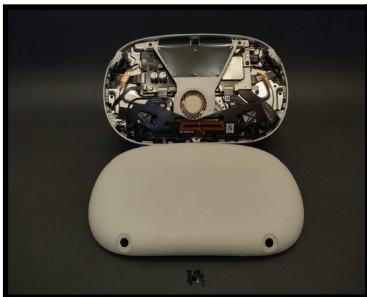
Figure 3.3 - Removal of the front cover.
