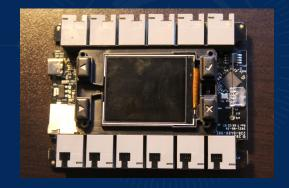
The device has 12 smart ports, a USB-C port for micro escape card storage, a radio antenna on the right, and an LCD screen for object display.
