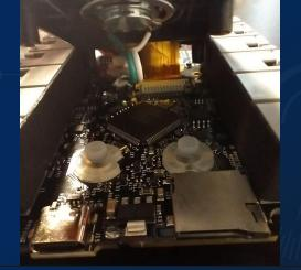
The LCD system includes a programming speaker, data storage chip, hotbar buttons, and an LCD screen connected to the display bus.
